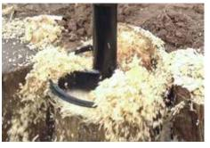
The unique pilot engages with the top surface of the tree stump drawing the tool down allowing the blades to engage with a clean horizontal cut.
