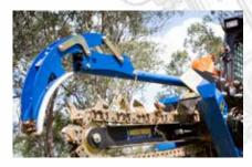
Our products incorporate many development features. The trench cleaner on our Trencher Attachments ensures a good clean cut with no residual spoil.
