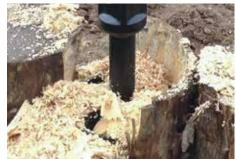
When the planer has achieved a deep cut, reposition to overlap the first hole and repeat the process until all of the stump is removed.
